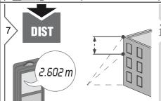
The result is shown in the main line and the measured distance above.
