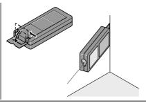
The orientation of the endpiece is automatically detected and the zero point is accordingly adjusted.
