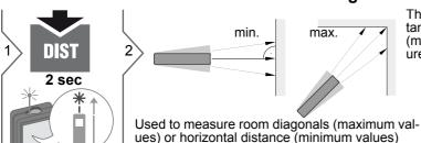
The minimum and maximum distance measured is displayed (min, max.). The last value measured is displayed in the main line.
