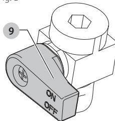
7. After the water has been drained, close the drain valve. The air compressor can now be stored.
