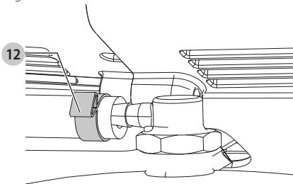
6. Remove three pump mounting screws securing pump.
